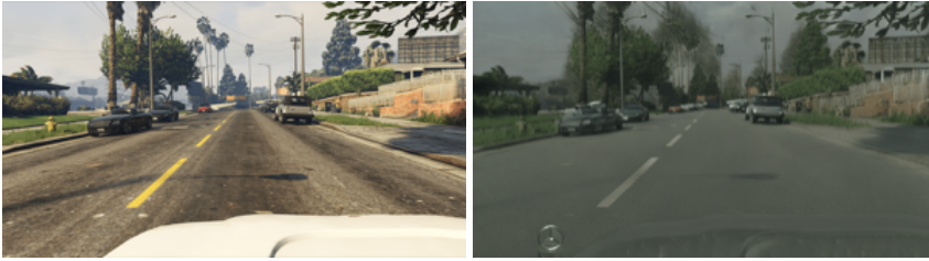
Fig. 4. Synthetic vehicle driving image (left) adapted to look realistic (right) [96].
