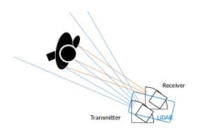
(a) LIDAR's working principle
