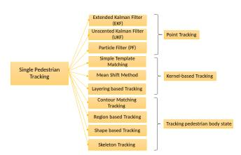
Fig. 7. Single pedestrian tracking models
