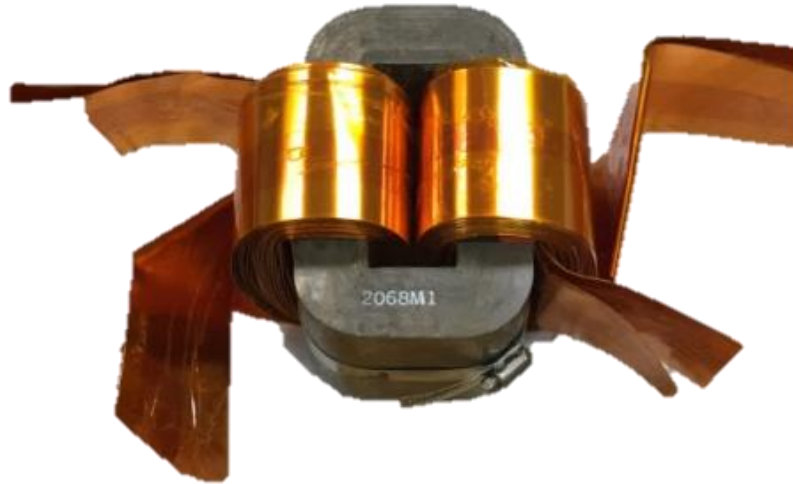
Fig. 9.2: Photograph of the fabricated high-frequency transformer for the S4T.
