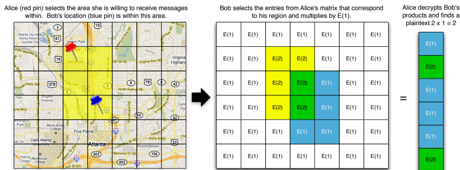
Fig. 1: Proximity Test Protocol. Alice builds a location matrix with encryptions of '1' in every entry except those that correspond to the area she is willing to receive tweets within. In her travel area, she enters encryptions of '2'. Bob selects the entries that correspond to his travel area, multiplies each entry by an encryption of '1', and returns the product to Alice. When Alice decrypts, she knows that: if any value is a '2', Bob's tweet is relevant to her. If every value is a '1', Bob's tweet is not relevant to her location.
