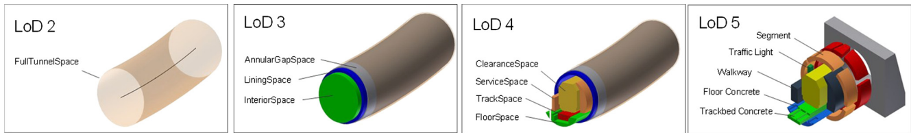
Fig. 2. A 3D representation of the LoDs 2–5 of the multi-scale shield tunnel product model [8].
