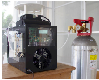
Fig. 10 Smart Trap for counting and classifying mosquitoes in real-time using optical sensor.
