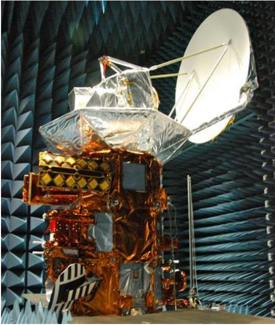
Figure 2: Aquarius in the deployed configuration during EMI/EMC testing
