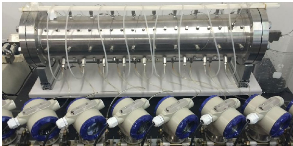
Fig. 4 Physical diagram of variable mass flow simulator of horizontal wellbore
