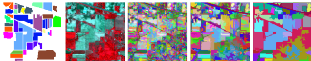
Fig. 1: The image representation of Indian Pines at different segmentation scales. From left to right: ground truth, false-color image, fine level (2486 regions), intermediate level (278 regions), coarse level (31 regions).
