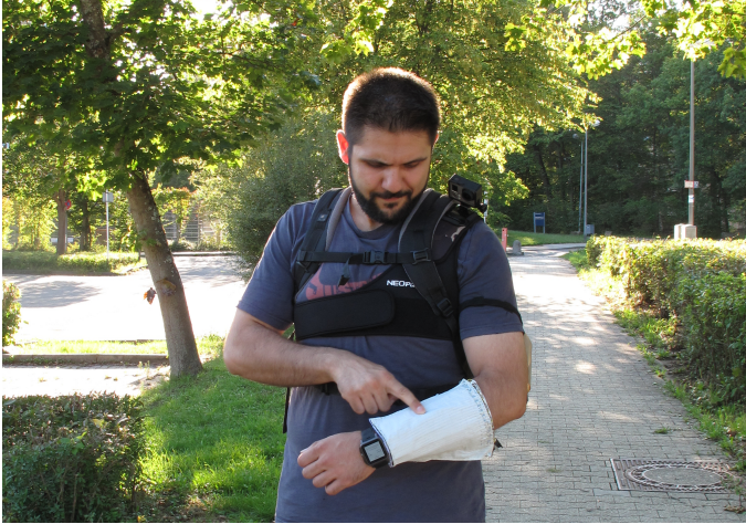
Figure 3.1: A user wearing the GestureSleeve at the forearm made out of touch-enabled textile. The GestureSleeve is capable of detecting gestures extending the input space of mobile devices.
