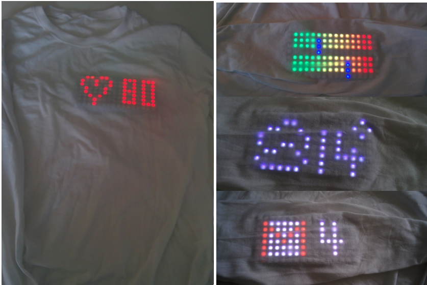
Figure 6.1: The wearable on-body display used in a t-shirt. The heart rate visualized on the chest (left) and a progress bar, weather information, and e-mail notification on the forearm (right).
