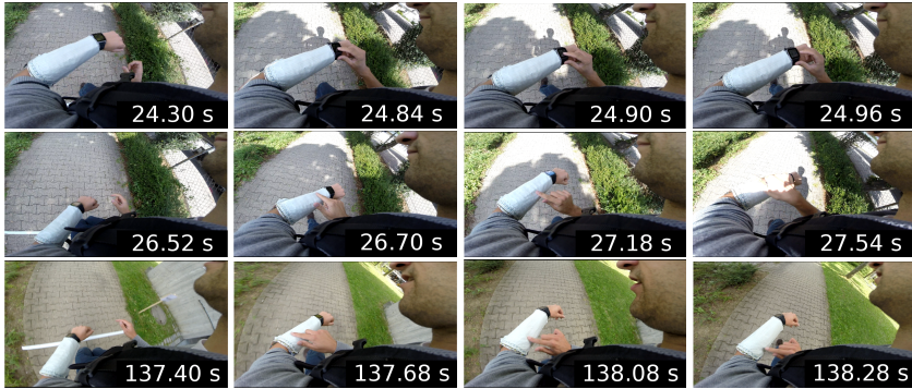
Figure 3.5: Video recordings of a user performing three different inputs. The user performs input on the smart watch using touch (top) and two different gestures on the GestureSleeve (middle and bottom).
