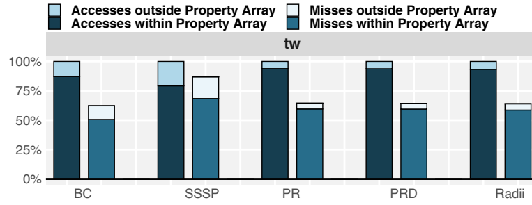
Figure 4.2: Classification of LLC accesses and misses (normalized to total accesses) for five graph applications when processing the tw dataset.
