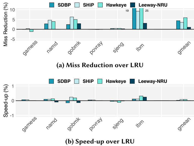
Figure 3.11: Evaluation of various cache management techniques for the No Opportunity SPEC CPU 2006 applications.
