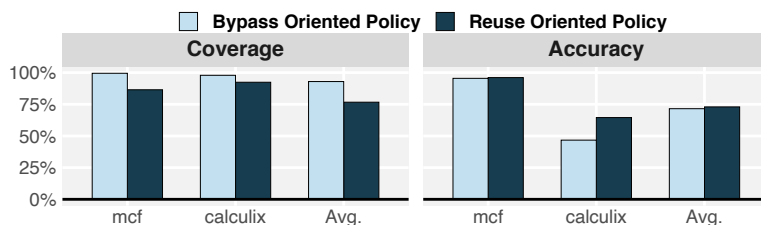
Figure 3.13: Prediction Coverage and Accuracy for Leeway-NRU static policies.
