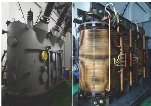
FIGURE 1. Photograph of three-phase oil-immersed transformer.
