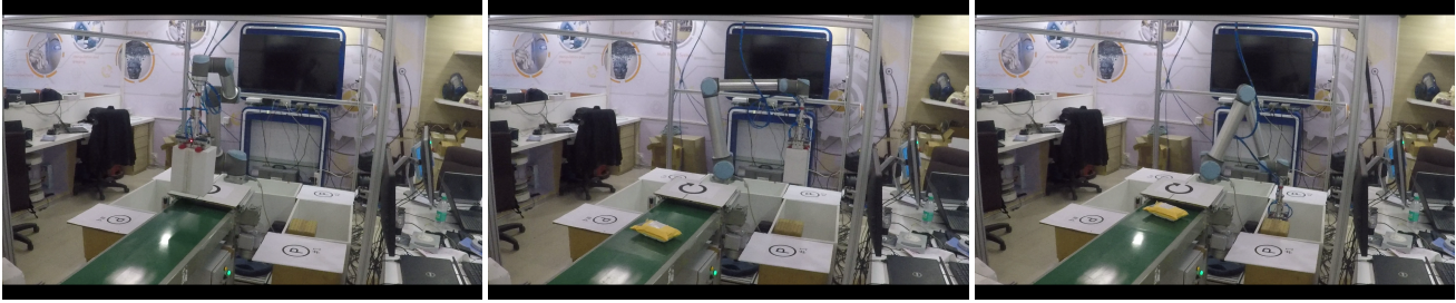
Figure 1: Prototype created in the lab. The conveyor belt brings single-sorted parcels with regular spacing. Demonstration of one pick and place cycle is shown, from left to right (a) Picking the parcel from the conveyor belt (b) Searching for the placement location (c) Placing the parcel inside the container.
