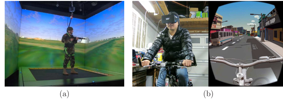
Figure 10.8: (a) An omnidirectional treadmill used in a CAVE system by the US Army for training. (b) A home-brew bicycle riding system connected to a VR headset, developed by Paul Dyan.
