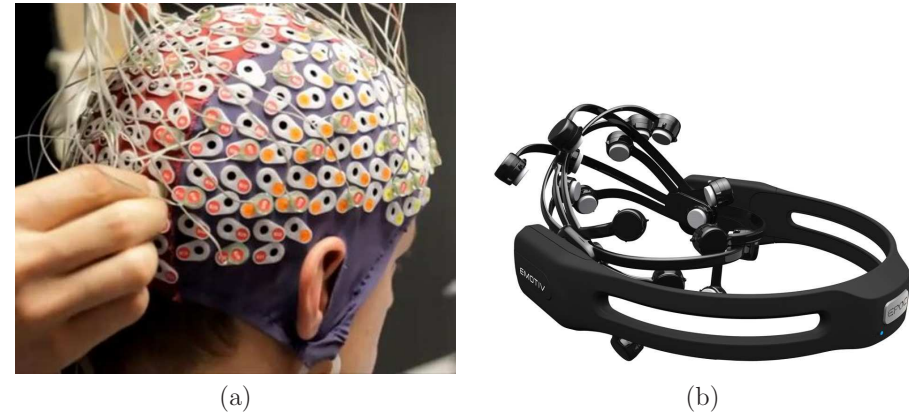
Figure 13.11: EEG systems place electrodes around the skull: (a) A skull cap that allows up to a few dozen signals to be measured (figure by Laboratory of Cognitive Neuroscience, EPFL, Switzerland). (b) Emotive wireless EEG device (figure by Emotiv and Emotiv EPOC+/Insight).
