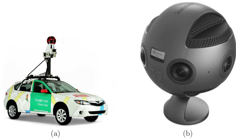
Figure 1.9: An important component for achieving telepresence is to capture a panoramic view: (a) A car with cameras and depth sensors on top, used by Google to make Street View. (b) The Insta360 Pro captures and streams omnidirectional videos.
