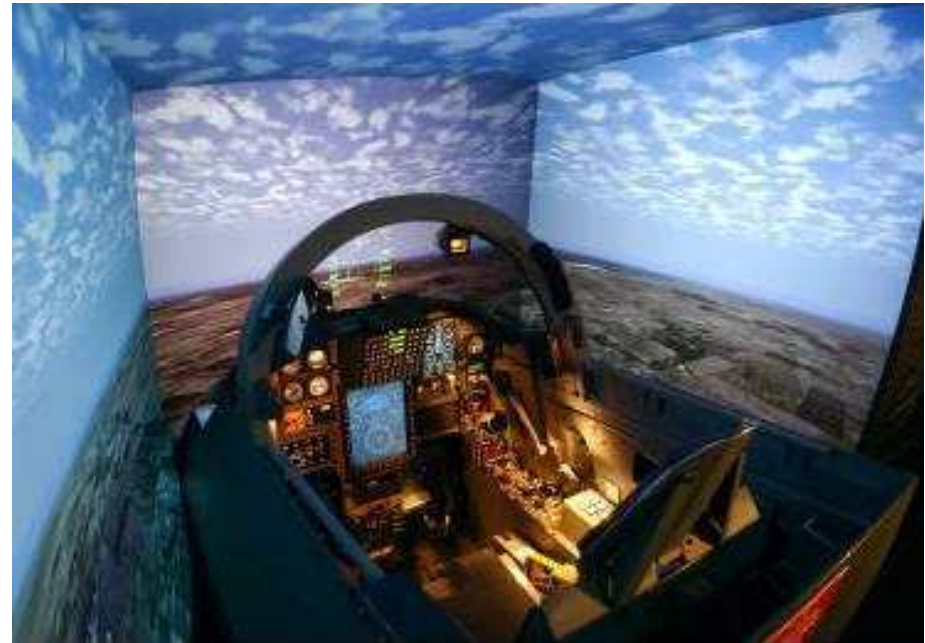
Figure 1.16: A flight simulator in use by the US Air Force (photo by Javier Garcia, U.S. Air Force). The user sits in a physical cockpit while being surrounded by displays that show the environment.
