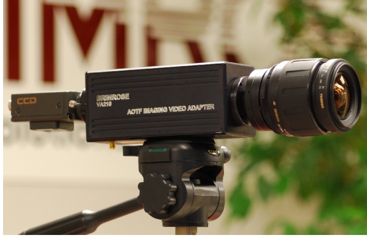
FIGURE 2.4: AOTF hyperspectral imaging system [1].
