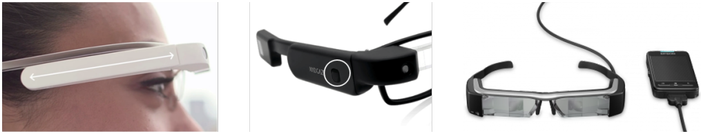
Fig. 6. Trackpad on spectacle frame (Left), Button (Middle), External controller wired with Espon smart glasses (Right)
