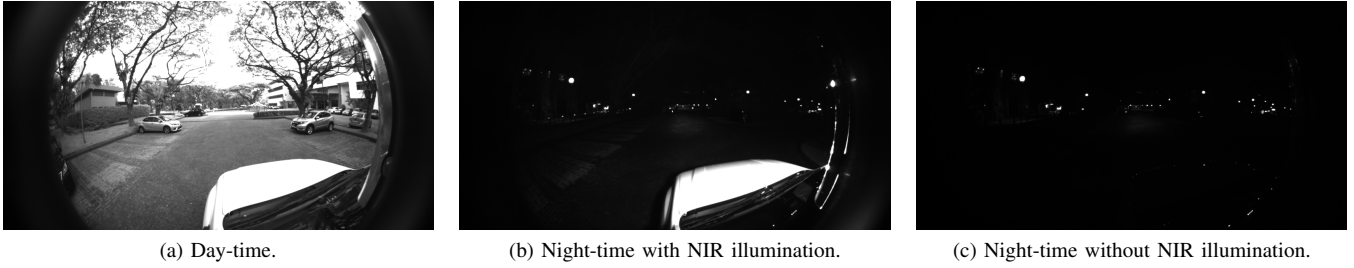
Fig. 4: Images captured from a front left camera on the AutoVision vehicle and in varying lighting conditions.
