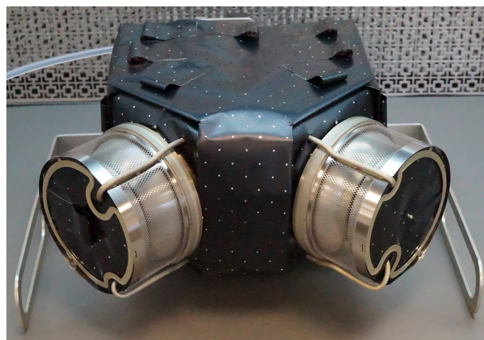
Fig. 4. Flight model of the SWA-EAS unit, showing the two orthogonally-mounted cylindrical electron optics subsystems attached to the control electronics box (which is housed beneath the black multi-layer insulation (MLI) blankets). The curved aperture deflector plates, lying either side of the apertures themselves, can be seen through the entrance grid on both heads.
