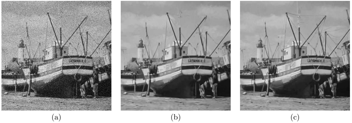
Figure 9: (a) The boat image corrupted by 20 dB of Gaussian noise and 10% outliers. (b) Denoising with BM3d (28.97 dB). (c) Denoising with joint KGARD-BM3D (31.52 dB).
