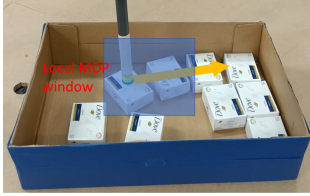
Fig. 3. Nested pushing of objects can rearrange several objects simultaneously and reduce the trajectory of the end-effector.
