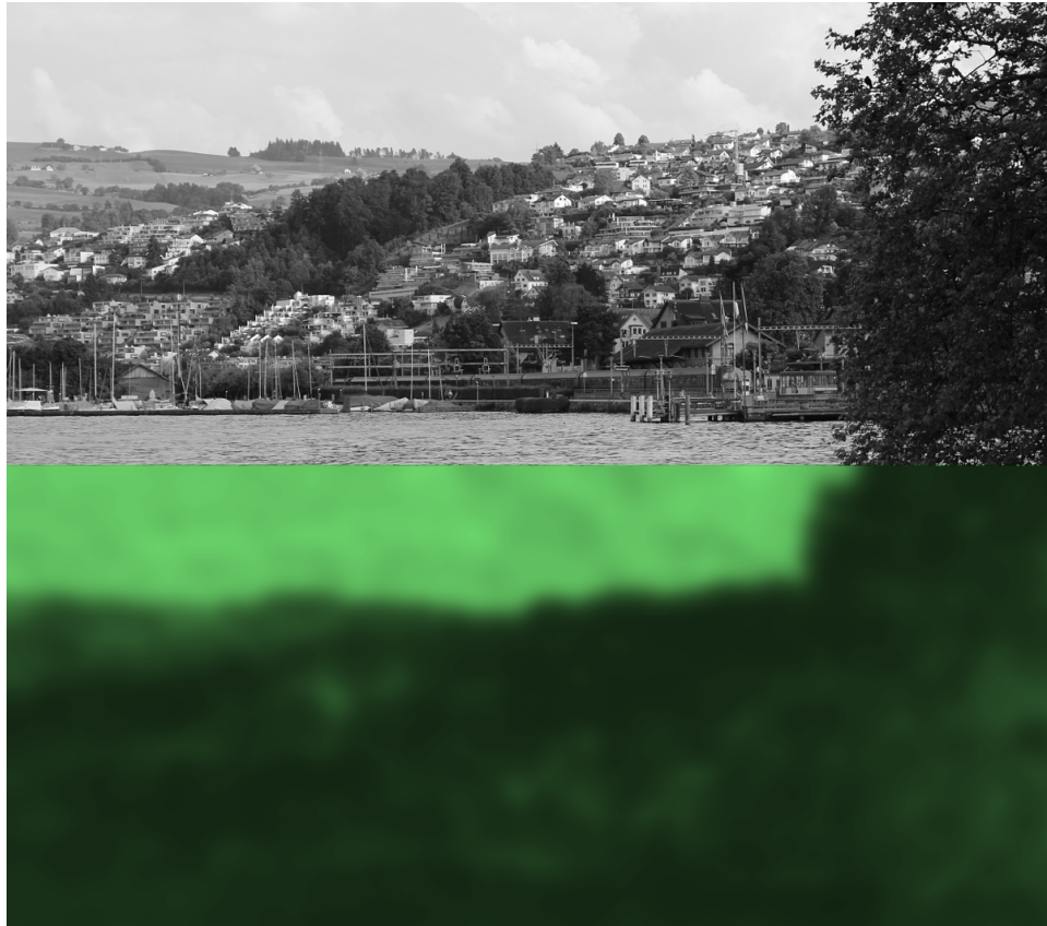
Figure 3: Landscape photo on the top with its visual mask shown on the bottom. Darker areas on the visual mask require less precise reproduction of details. Visual masking allows areas of the photograph to be stored at different accuracy, up to 6\times quantization difference for this image. According to this visual masking model, the sky needs to be compressed with less loss than the tree, lake and the buildings for a uniform experience of compression quality. Guetzli computes two separate masking models – one for low spatial frequency color modeling and one for high spatial frequency color modeling. Both models contain one mask for each dimension of the color space. The mask above is the high spatial frequency intensity mask.
