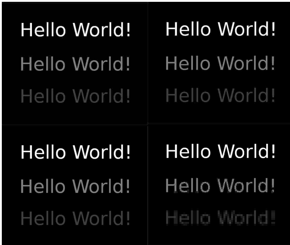
Figure 5: The top part of the figure shows how imagemagick convert --subsample-factor 1x1 stores the blue channel of the image in Figure 2. One can observe that the blue channel, which is displayed here as a grayscale image, is stored with similar accuracy in the black area and in the yellow area.
