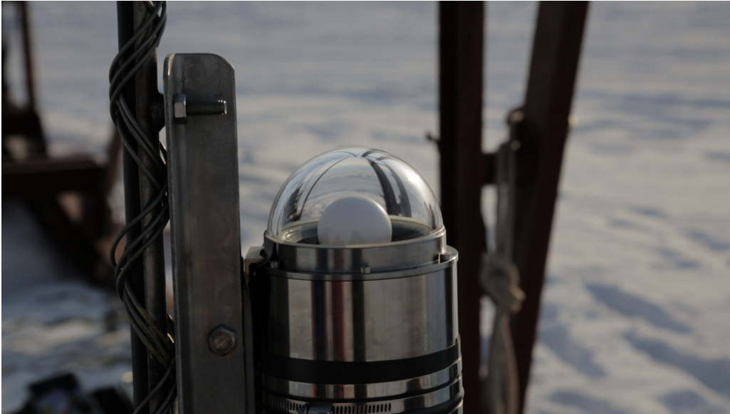
Figure 3: The POCAM module mounted to the GVD string before deployment in the Baikal lake.
