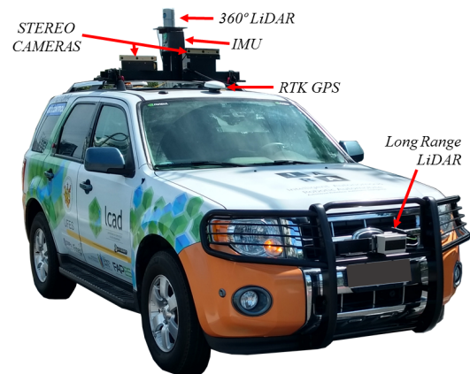
Figure 14: Intelligent and Autonomous Robotic Automobile (IARA) that was the first Brazilian self-driving car to travel autonomously 74 km on urban roads and highways. A video that shows IARA operating autonomously is available at https://youtu.be/iyKZV0ICysc .
