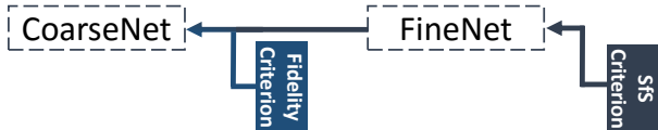
Figure 7: Criterion flow. Gradients from both loss criteria are propagated back to CoarseNet.
