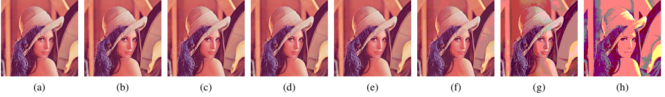
Figure 8: Influence of color reduction: (a) without color reduction; (b) to (h) with color reduction, starting with only one bit in the red, green, and blue channel put to zero for (b) up to seven bits for (h).
