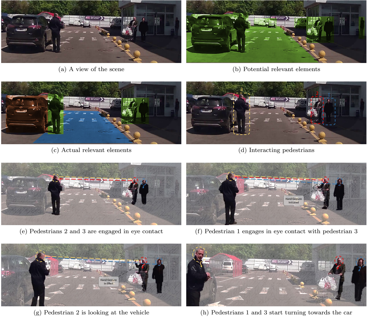
Figure 40: Joint attention and nonverbal communication in a traffic scene. In sub-figure c colors indicate the priority of attention, from highest to lowest: green , blue , yellow and red .
