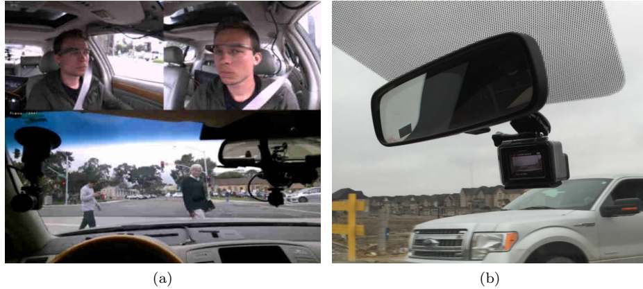
Figure 15: Examples of using technology for behavioral studies: a) eyetracker for driver behavior analysis [139], and b) the placement of a concealed camera for naturalistic traffic recording.
