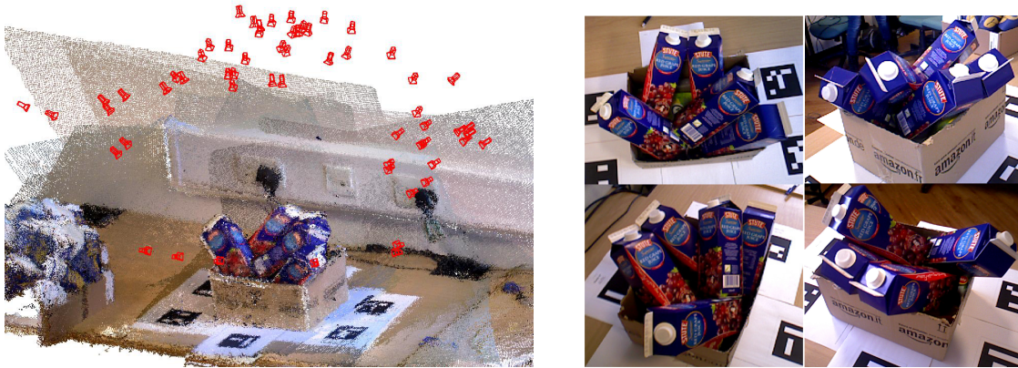
Figure 3.11: (left) Accumulated view and camera pose of different views of a pile of juice box scenario; (right) images from four different views.
