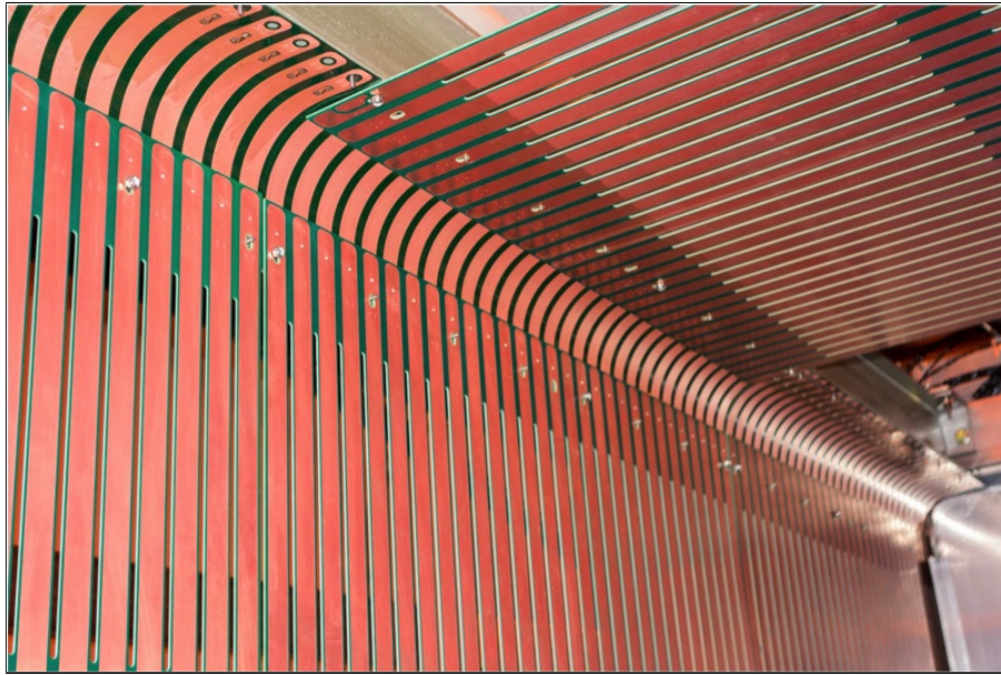
FIG. 34: A photo of the 35 ton LBNE prototype field cage.
