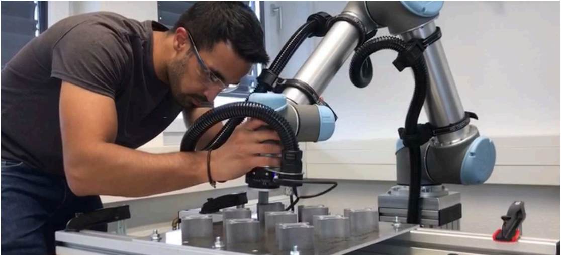
Figure 2.5.: Kinesthetic teaching for the peg-in-a-hole problem with a UR5 robot arm.
