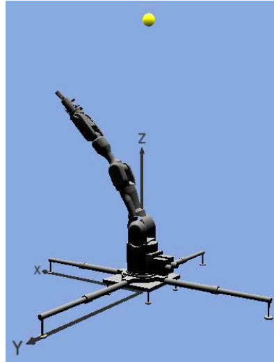
Figure 4.2.: Visualization of the simulated Mitsubishi PA-10 throwing a ball.
