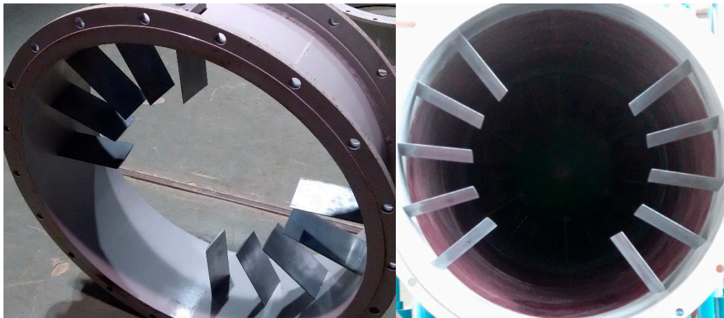
Figure 2. Blade-type swirl distortion generator.
