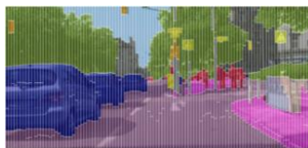
Fig. 1: Semantic stixel representation where the image is segmented into drivable road, sky, and vertical "sticks" (Schneider, 2016).
