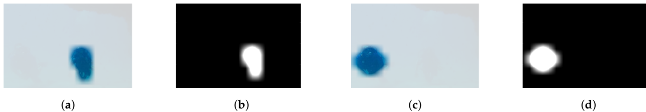
Figure 4. Example of attended locations computed from the original image depicted in Figure 3: (a) attended location deriving from center-surround operations on intensity between scales \sigma = 3, 6 and (b) corresponding attended mask; (c) attended location deriving from center-surround operations on intensity between scales \sigma = 4, 7 and (d) corresponding attended mask.
