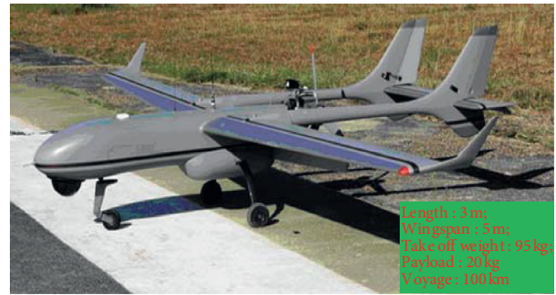
FIGURE 3: UAV and its main constitute parameters.
