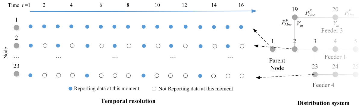
FIGURE 2. Temporal resolution of measurements associated with different nodes.
