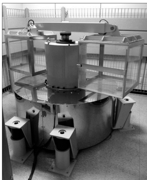
Figure 1. Gravity Simulator for the research on hypergravity [2].
