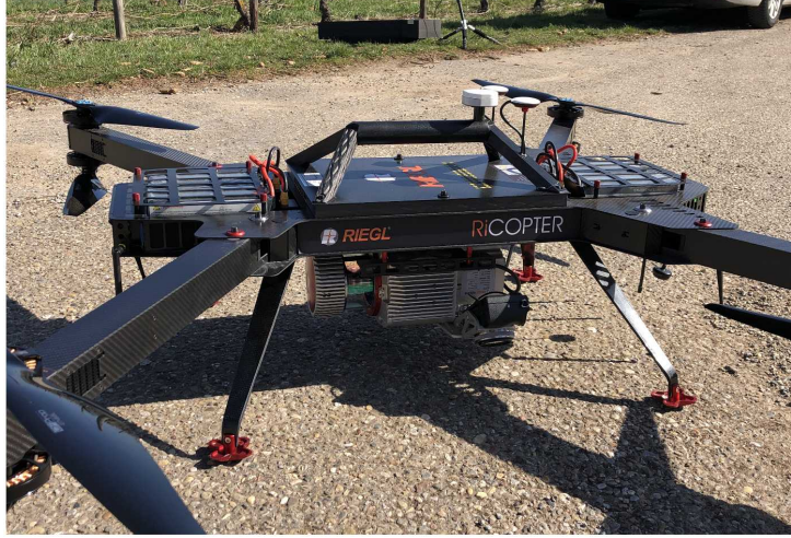
Figure 2: Ricopter platform equipped with Riegl VUX-1LR scanner and two oblique Sony Alpha 6000 cameras used for capturing H3D.
