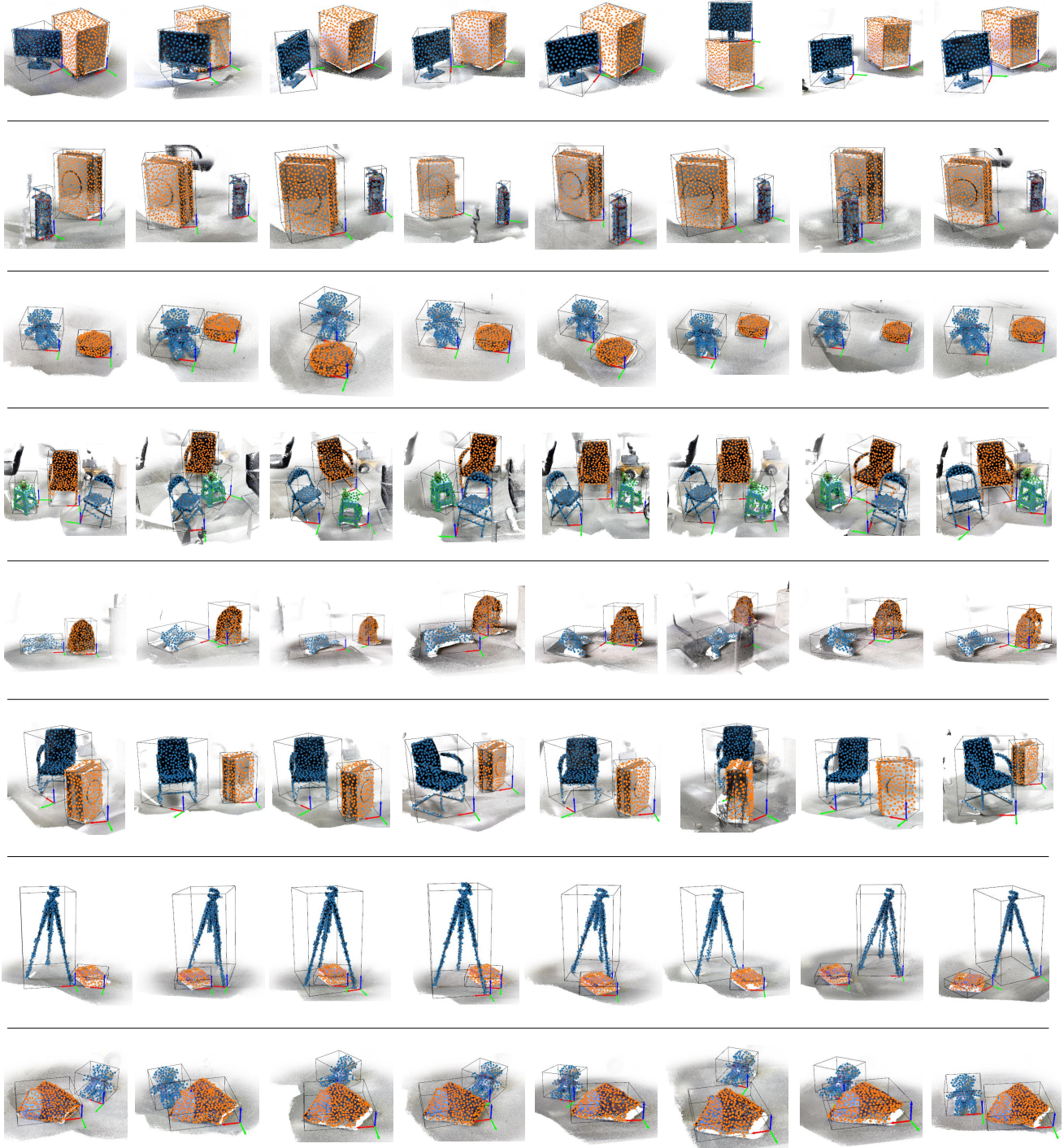
Figure S12. Visualization of the DynLab dataset. Each row shows 8 different dynamic configurations of the same set of rigid objects. Annotated bounding boxes are parallel to the ground plane and reflect the objects' absolute poses.
