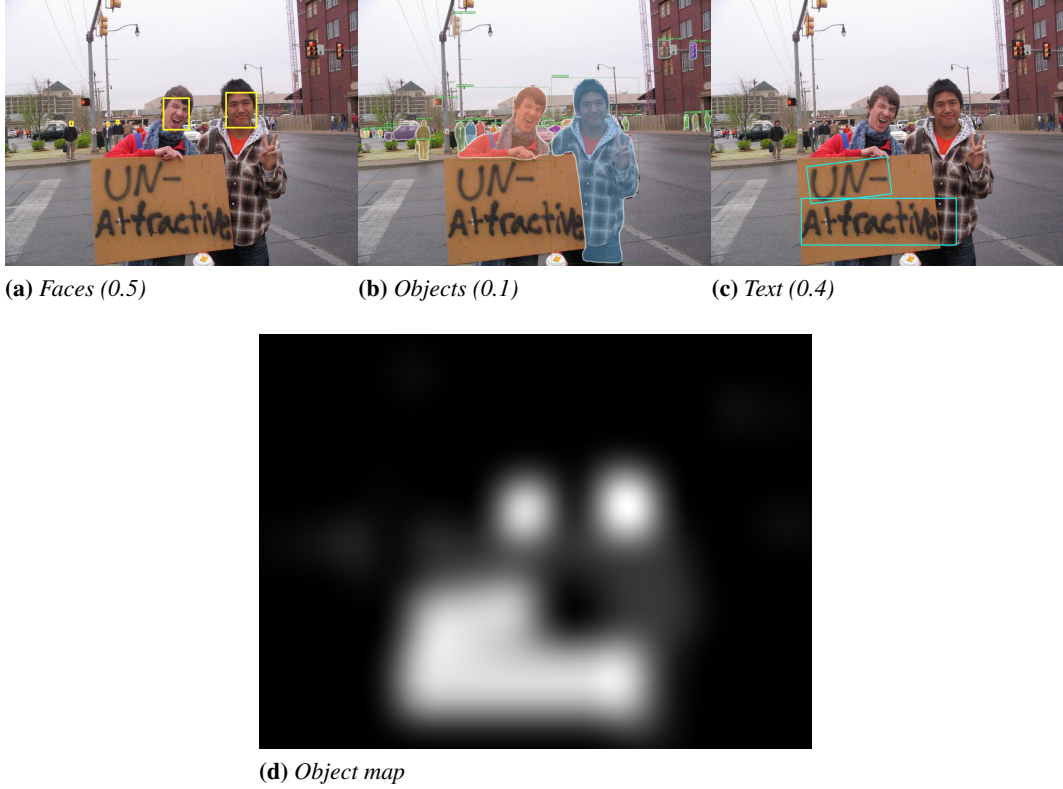
Figure 2.10: Components of the object map: (a) shows the result of the face detector module; (b) the result of the object segmentation; (c) text detection result. In brackets, the weights of each component, in terms of contribution to the final object map (d).
