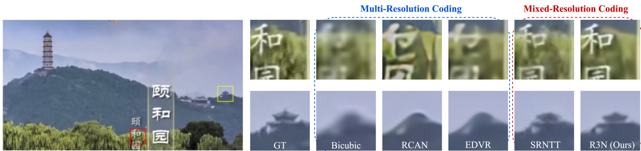
Figure 1: A comparison of visual quality on low-resolution compressed video restoration (reconstructing 1080p results from 270p compressed videos). RCAN [49], EDVR [41], SRNTT [51] are the state-of-the-art methods for single image, video and reference-based super-resolution, respectively. In this paper, bicubic, RCAN and EDVR are used in the multi-resolution coding pipeline; SRNTT and the proposed R3N are used in the mixed-resolution coding pipeline.
