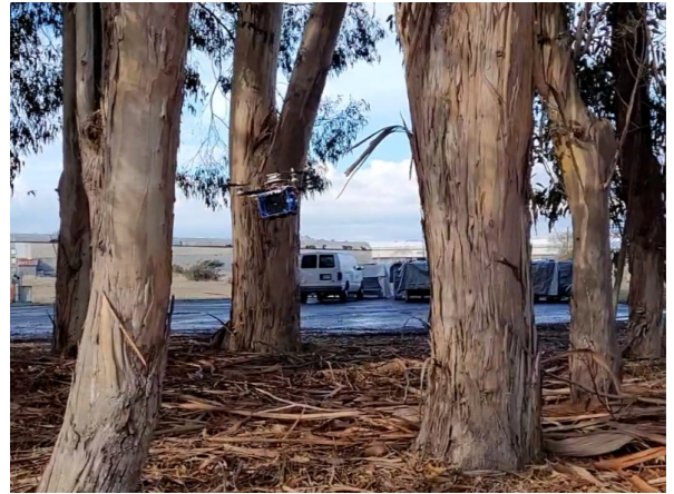
Fig. 1. The vehicle flies autonomously using visual-inertial odometry and the collision-avoidance planner through a forest, avoiding trees.
