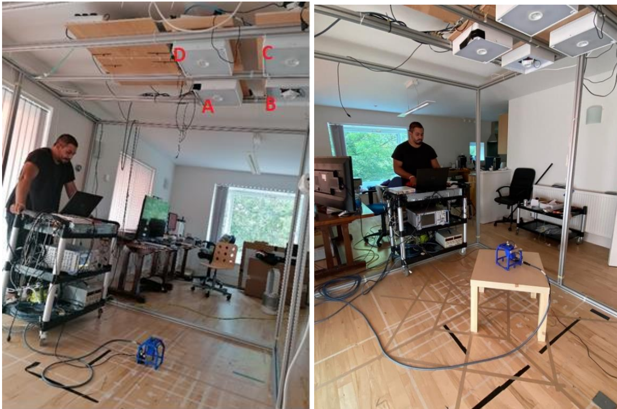
Figure 4: Taking mmWave measurements at ground level with RLHs labelled A, B, C, D and at 0.7 m above ground
