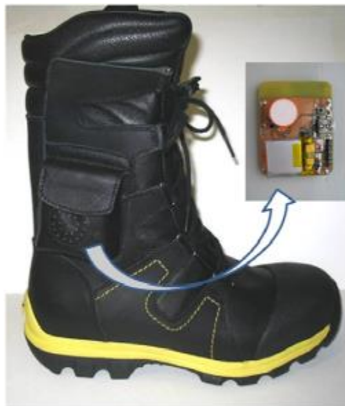
Figure 35 Firefighter's boot with built-in pocket used for enclosing the CO 2 sensor and wireless sensing module (on right) 83
