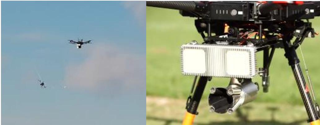
Figure 70 Fortem DroneHunter in action (left); radar mounted on the drone (right)
