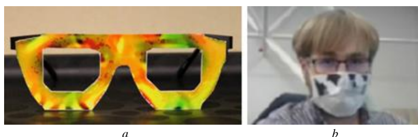
Fig. 12. Ways to perform adversarial attack: a – sunglasses with an adversarial print [55]; b – medical mask with especially crafted black spots [56]
