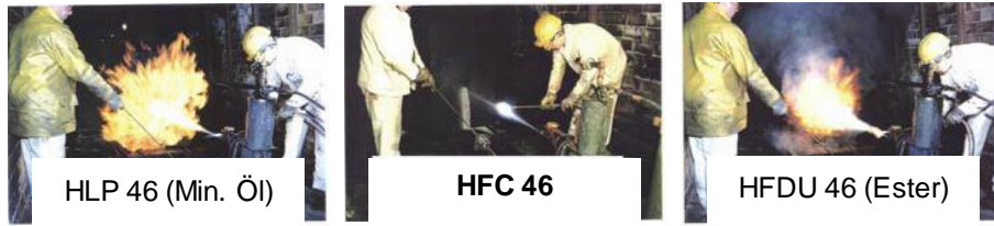
Fig. 1 Ignition tendency comparison for HFC and conventional hydraulic oils.
