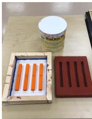
Fig. 1 The rapid prototyping tool for making the tensile bars.
