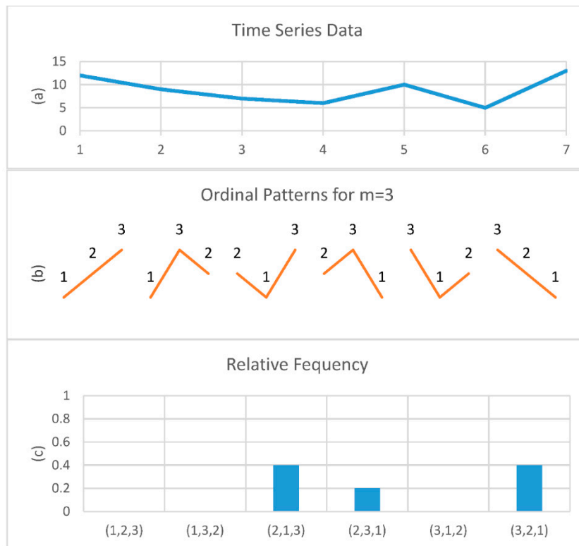
Figure 3. Example of permutation entropy estimation. (a) Time series X = (12, 9, 7, 6, 10, 5, 13) . (b) The six possible permutation patterns for m = 3 . (c) The relative frequency of all possible ordinal patterns for n = 3 for this time series, P(2,1,3) = 0.4 , P(2,3,1) = 0.2 and P(3,2,1) = 0.4 .
