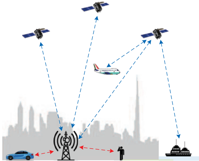
Figure 25 (Color online) Integration of terrestrial and satellite communication networks.
