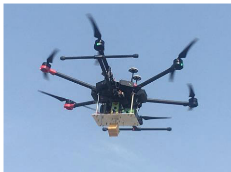
FIGURE 12. W band mini-SAR prototype on a multi rotor UAV platform.
