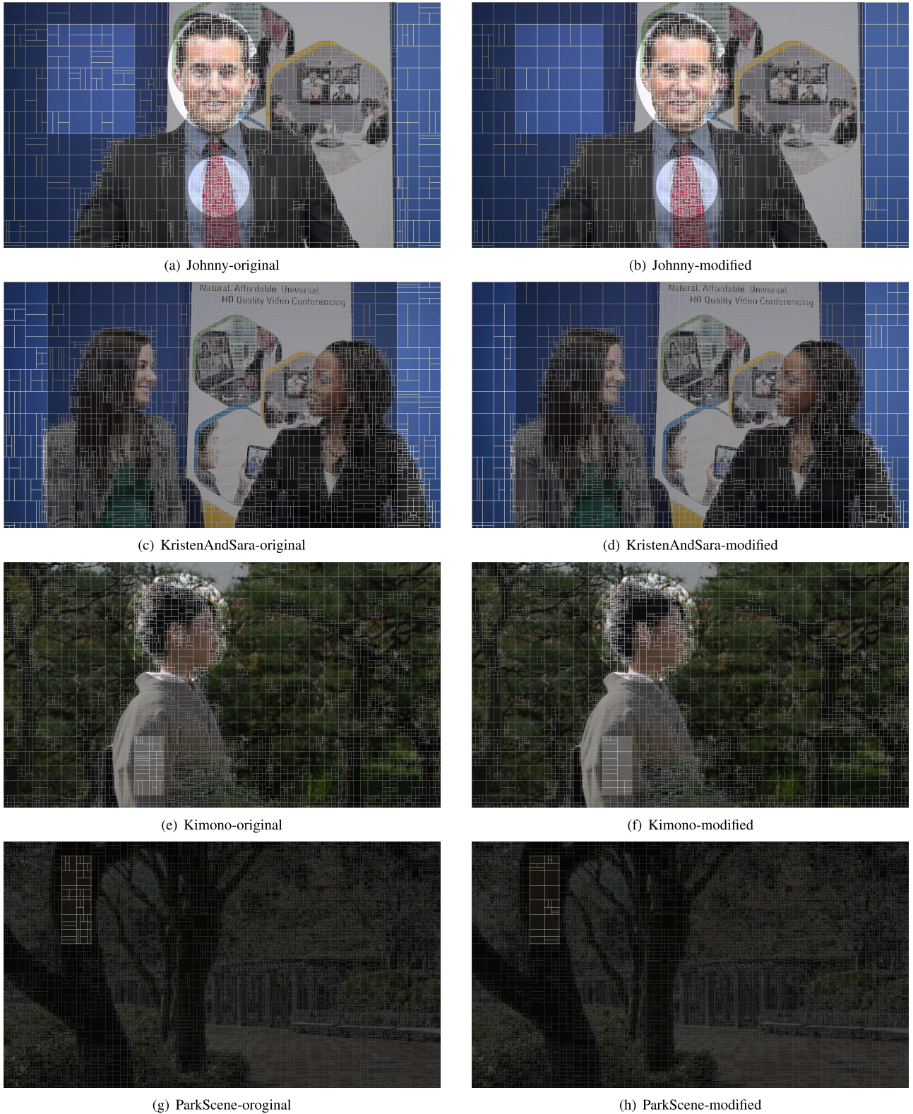
FIGURE 6. Comparison between the original (left) and modified (right) CU partition structure when QP equals 27. The labeled rectangular areas are processed by the pruning strategy while the circular regions maintain a sophisticated block partition structure.
