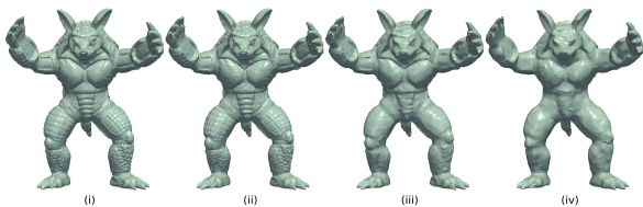
FIGURE 4. Compact representation of the Armadillo geometry using a different number of eigenvectors of the graph Laplacian: (i) original geometry, (ii) compact representation using 90% (those that correspond to small eigenvalues) of the eigenvectors (iii) compact representation using 25% of the eigenvectors (iv) compact representation using 10% of the eigenvectors. Note that the surface attains more high-frequency detail as we increase the number of eigenvectors.
